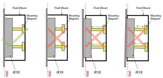
The device is suitable for use in dry interior rooms and can only be mounted on a standard-sized round or square wall flush mounting box. The iX10 should be mounted only after the wall painting is completed to avoid damaging the product's appearance. Important considerations for mounting are listed below
