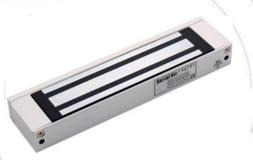
The magnetic lock is designed for wooden door, glass door, and steel door with the opening angle of 90°. The maximum thrust of the lock is 272 kg (599.8 lbs). It can be used for controlling door opening/closing, and the indicator shows the door status. It supports signal output of door lock output status testing.
